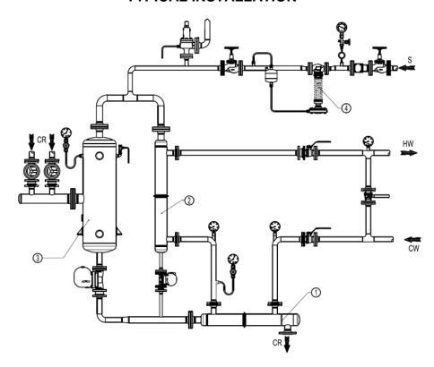
The condensate return (CR) is expanded on a flash vessel (3). The flash steam which is produced there and the remaining condensate are then directed to the respective heat exchangers (1 e 2) where, in the meanwhile, the pressurized feed water (CW) is heated (HW) before it passes to the economizer or is directly introduced in the steam boiler (it is recommended to install a by-pass from CW to HW).
